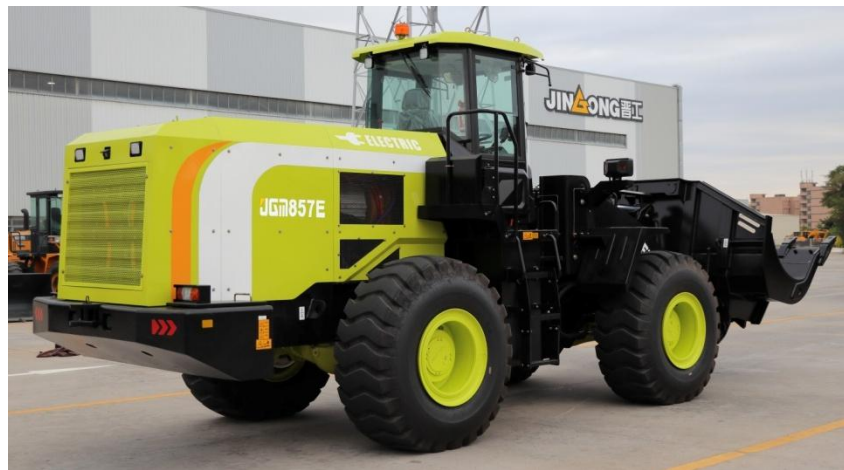
Jingong's first-generation 5.5-ton electric loader, with a battery of 210KWh.
