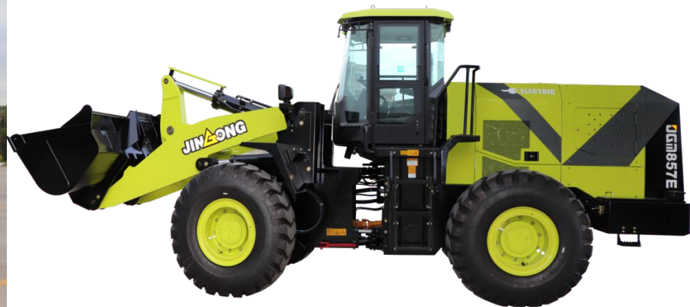
Jingong's second-generation 5.5-ton electric loader, The battery uses a configuration of 351KWh, At the same time, the shortcomings of the first-generation products are optimized.
