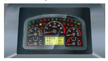
The combination instrument includes five analog instruments, plurality of colorful indicator lights an LCD screen. Through this intuitive system, the operator can monitor whether the system is working properly.
