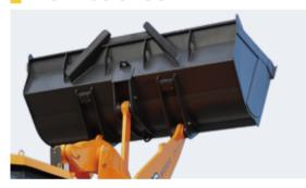
The new bucket with enlarged side plates which make the structure more firm and reliable, and more convenient to load; The heightened rear plate can prevent spillage of materials during hopper collection; The adjustable bucket limit ensures that both sides of the bucket limit block and the boom plate are close tight during withdraw bucket, thus shortening the cycle time; ear-resistant gaskets are added to each pin shaft of the working device to reduce shaking.
