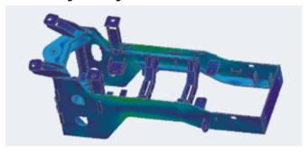
The wheelbase extended to 3300mm, and the rear suspension distance is increased. The front and rear axle load distribution are more reasonable and stability. The reliability of the frame is greatly improved through finite element simulation analysis.
