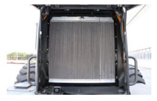
Use single-layer parallel design, The radiator of the water tank and the oil radiator of the torque converter are air cooling, and the hydraulic oil radiator is water cooling.
