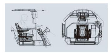
Through the man-machine engineering simulation design, the operating parts such as the operating handle, steering column, and switch keys commonly used by drivers are mainly considered to improve the comfort and convenience of operation.
