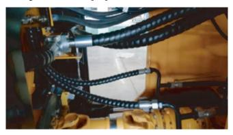
The centering arrangement of the rubber hose reduces the connection between the rubber hose and the steel pipe, more easy to maintenance and reduces the failure rate.
