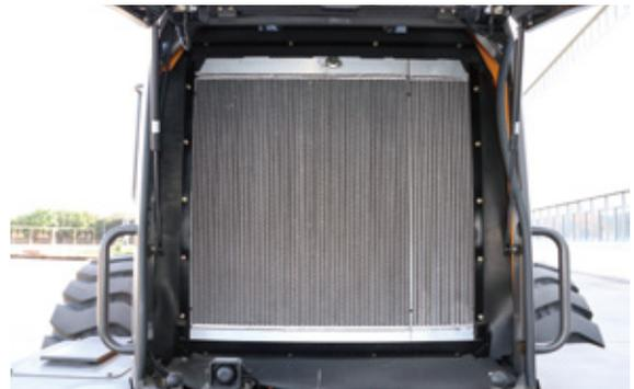
Use single-layer parallel design, The radiator of the water tank and the oil radiator of the torque converter are air cooling, and the hydraulic oil radiator is water cooling.
