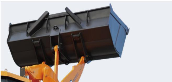
The new bucket with enlarged side plates which make the structure more firm and reliable, and more convenient to load; The heightened rear plate can prevent spillage of materials during hopper collection; The adjustable bucket limit ensures that both sides of the bucket limit block and the boom plate are close tight during withdraw bucket, thus shortening the cycle time; ear-resistant gaskets are added to each pin shaft of the working device to reduce shaking.
