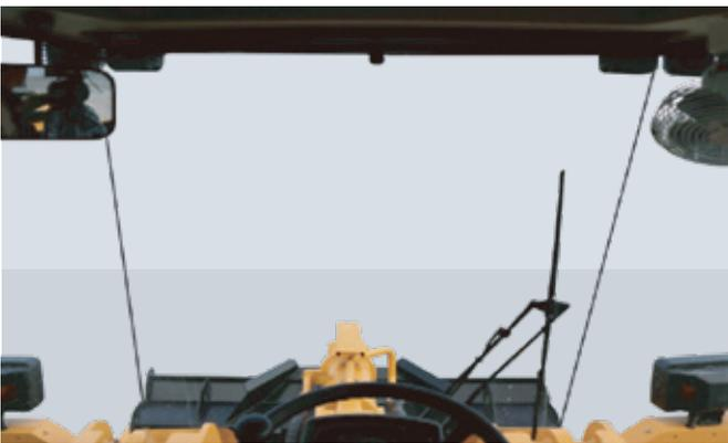
The front hyperboloid tempered glass with panoramic view, the right window is equipped with a glass frame that can be pulled up and down, enlarged inside and outside rearview mirror, freely adjust the sun shade and standard equipped with AC, to provide a wider and more comfortable operating environment and vision for the driver.
