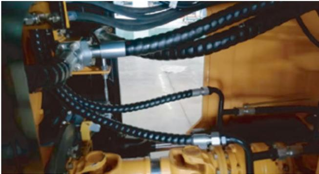
The centering arrangement of the rubber hose reduces the connection between the rubber hose and the steel pipe, more easy to maintenance and reduces the failure rate.
