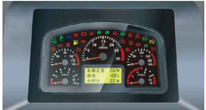
The combination instrument includes five analog instruments, plurality of colorful indicator lights and LCD screen. Through this intuitive system, the operator can monitor whether the system is working properly.
