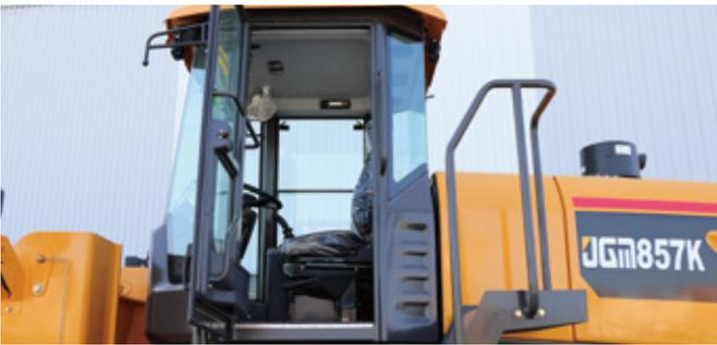
Widened cab door without threshold makes it easier to clean up sundries in cab; With handrails on both sides, it is convenient for operators to get in and out of the cab.
